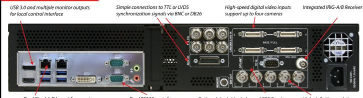
Dual Gigabit Ethernet for remote control and streaming video
