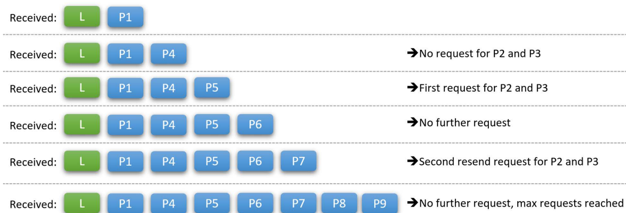
Figure 38: Controlling the resend of packets
